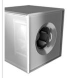
The housing supporting frames are double chamber aluminum profiles with corners made of plastic and double skinned (20mm) galvanized steel panels insulated with non-inflammable, noise and temperature insulating fiberglass mats. One side of the casing is open as standard.
