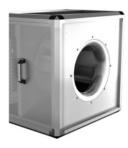
The housing supporting frames are double chamber aluminum profiles with corners made of plastic and double skinned (20mm) galvanized steel panels insulated with non-inflammable, noise and temperature insulating fibreglass mats. Outlet and side panel can be changed. A drip tray is included as standard in base and connections provided with blind plugs. The matching condensate drain connection is KAS.1 (supplied loose) included and can be easily mounted to the mounting holes if necessary.
