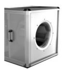
The housing supporting frames are double chamber aluminum profiles with corners made of plastic and double skinned (20mm) galvanized steel panels insulated with non-inflammable, noise and temperature insulating fibreglass mats. Outlet and side panel can be changed. A drip tray is included as standard in base and connections provided with blind plugs. The matching condensate drain connection is KAS.1 (supplied loose) included and can be easily mounted to the mounting holes if necessary.
